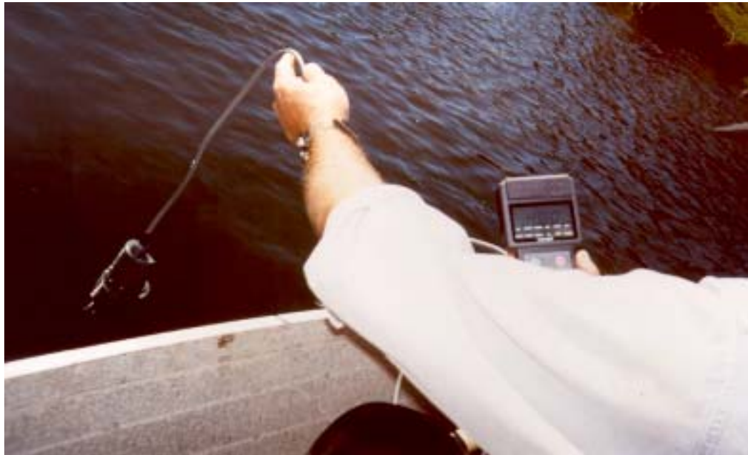
Figure 2: The multi-parameter probe in use. The transducer is slowly lowered into the water to known depths, and water conductivity (viz. salinity) is recorded from the LCD display readout.
