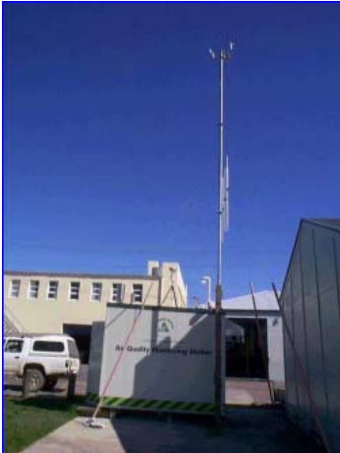
Figure 3.2: Birch Lane air quality monitoring station
