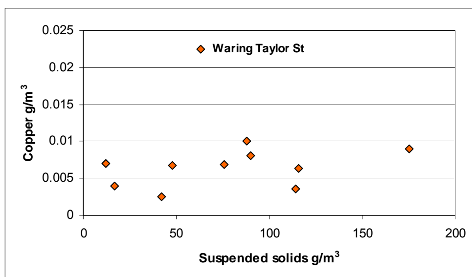
Fig. 5.5: Copper and suspended solids in Wellington stormwater.
