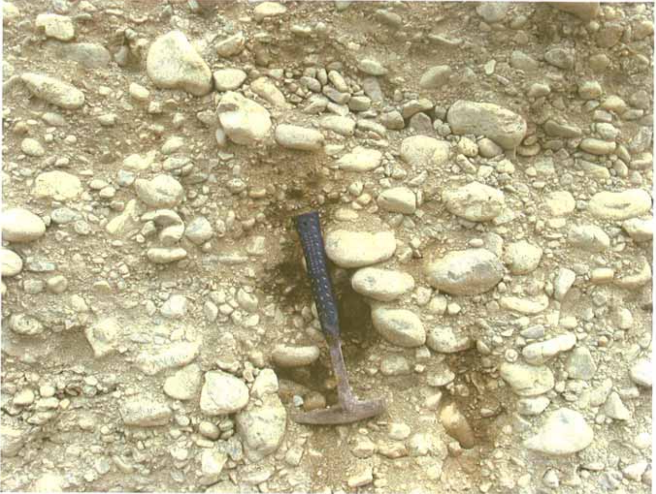
Figure 6: Typical In-Situ Profile of Gravel, Cobbles and Sand Forming Cut Slope in Old Excavation
