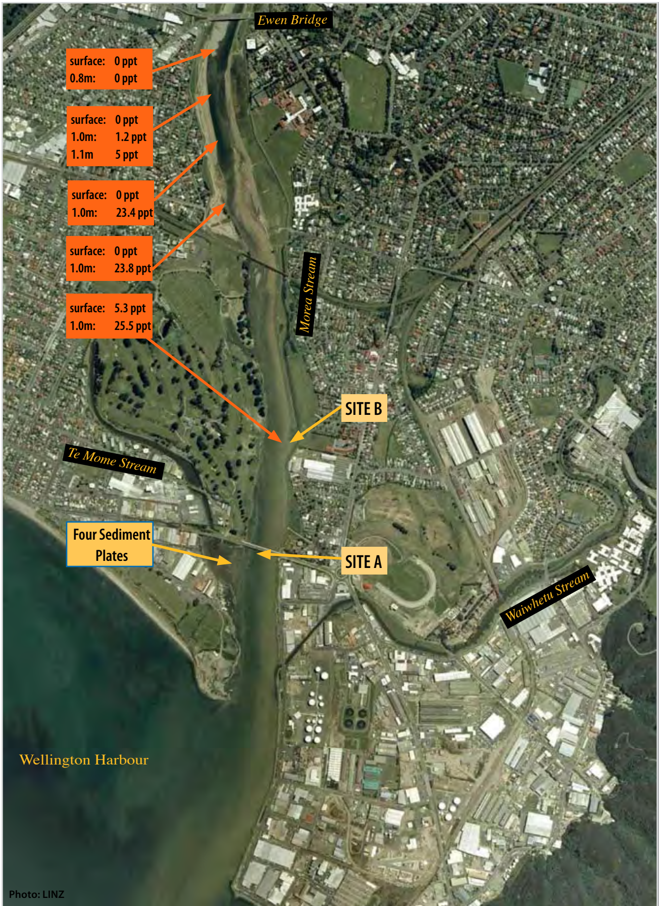
Figure 2. Hutt River Estuary Site Locations and Salinities, 21 January 2010. MHWS 10.45am. Salinity measured between 10.30-10.50am. Water temperature: 18.5°C above rail bridge, 19.4°C at lower site.
