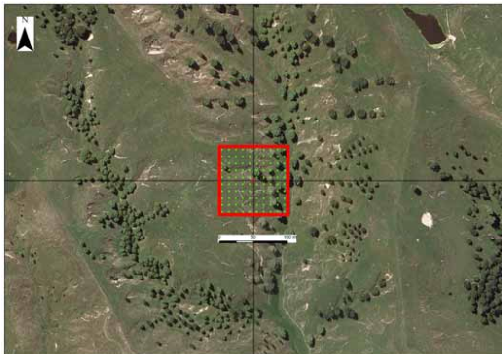
Figure 2.4: Soil stability monitoring site, showing the 100 dot grid used to calculate the amount of bare soil
