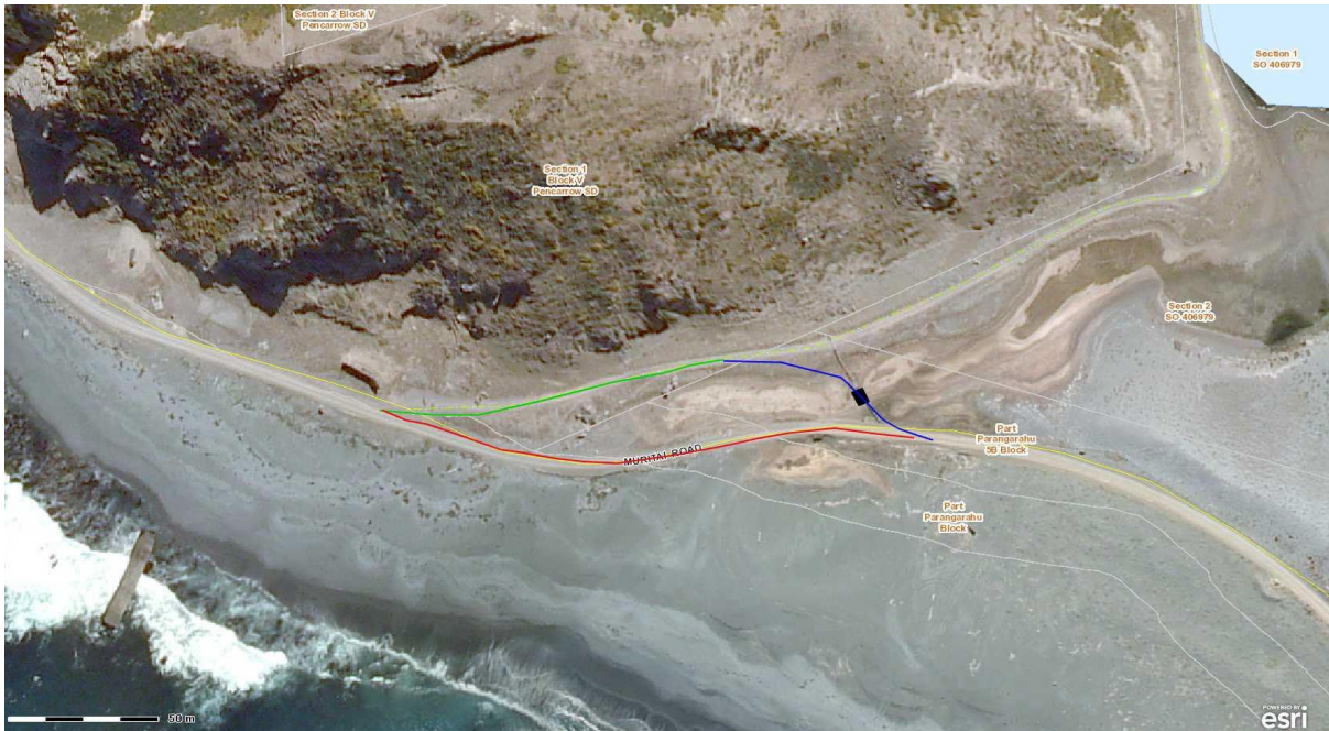
Figure 4. Proposal for road realignment at the mouth of Lake Kohangapiripiri to restore natural breaching of the lake and assist fish passage. The existing perched culvert can be seen adjacent to the existing road. Red line is road to be removed, blue line is new road, green line is existing road to be upgraded. Black rectangle is proposed new box culvert. Image courtesy of Tim Park.
