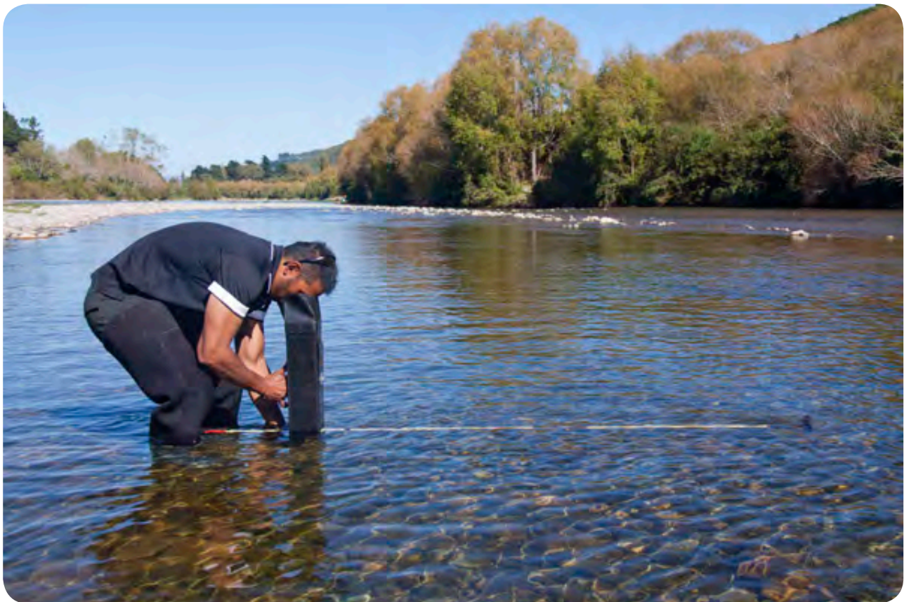
An assessment of water clarity on the Hutt River at Silverstream. A black disc fixed at 1.6 m from the viewer is used to assess whether the water clarity guideline is being met
