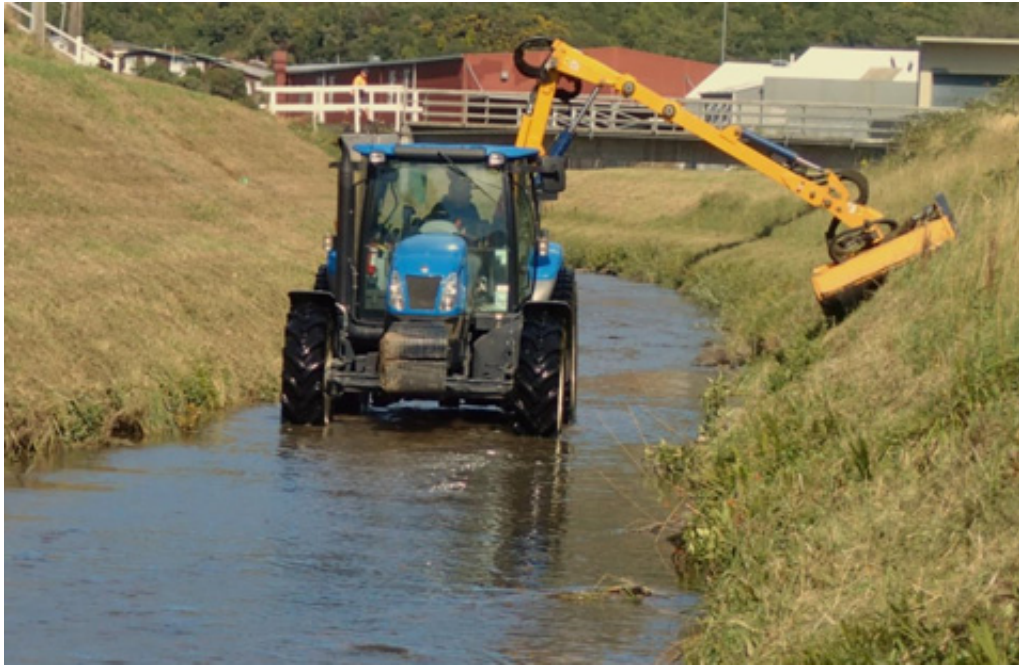
Figure 3.2: A tractor in Porirua Stream on 13 February 2013 mowing the stream banks approximately 1 km upstream of our monitoring site. Turbidity peaked at 12.4 FNU during the eight hours it was elevated
