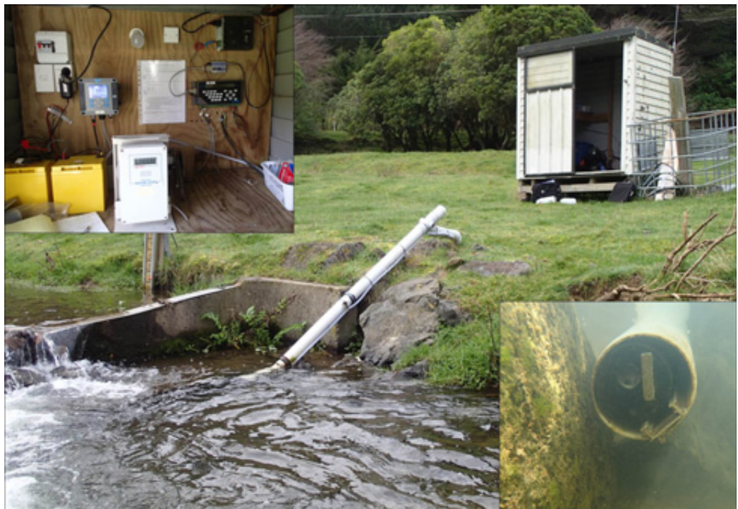
Figure 2.3: Horokiri Stream at Snodgrass site with insets of the SC-200 control unit and logger setup (top left) and in-stream turbidity sensor (bottom right)
