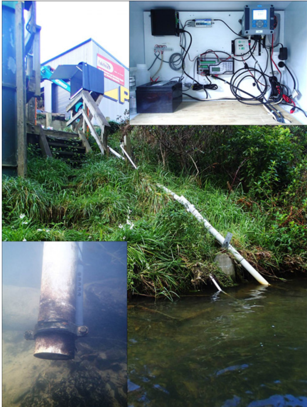
Figure 2.4: Pauatahanui Stream at Gorge site with insets of the SC-200 control unit and logger setup (top right) and in-stream turbidity sensor with auto-sampler intake hose attached to sensor housing (bottom left)
