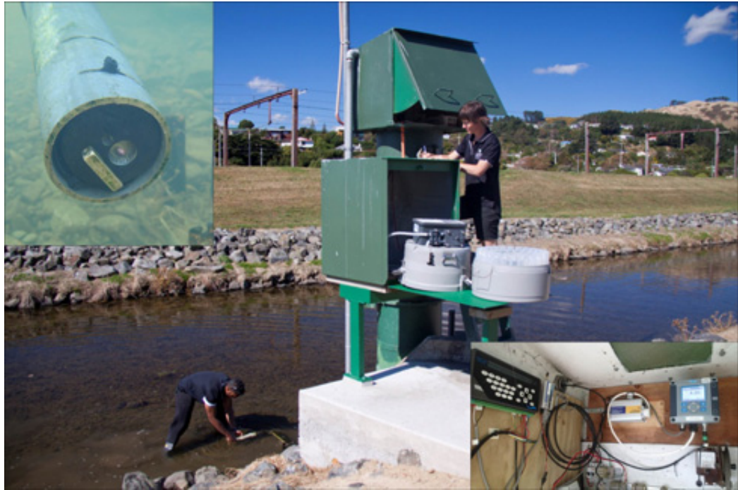
Figure 2.2: Porirua Stream at Town Centre site. Top left inset: Turbidity sensor in the stream with lens and wiper showing. Bottom right inset: SC-200 control unit (top right) and logger (top left) setup
