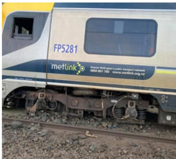
Figure 1. FP5218 derailed and pantograph overextended
