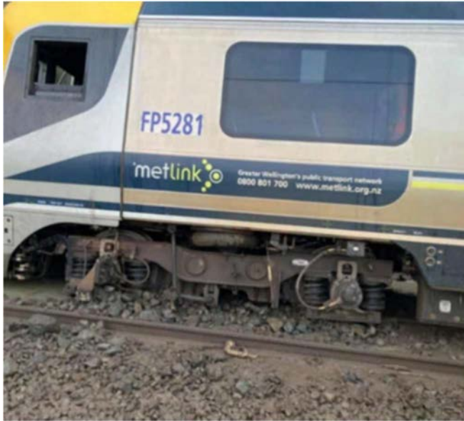
Figure 1. FP5218 derailed and pantograph overextended
