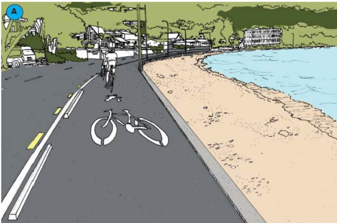
A. Looking south at Lowry Bay, just south of the red bus shelter, showing a dwarf cantilevered wall and 2.5m shared path.
