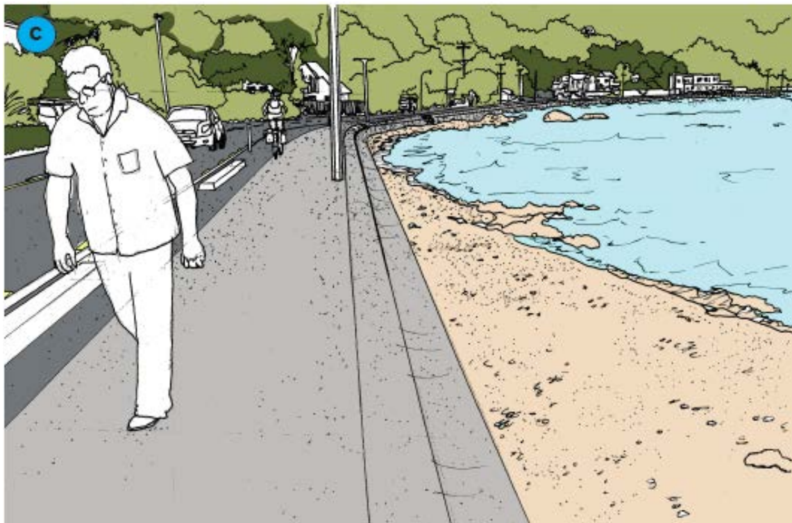
C. Looking south at Mahina Bay, showing a new 3.5m width double curved sea wall.
