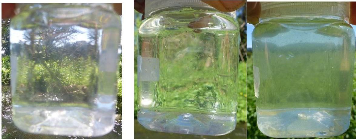
Photo A6: Water clarity in Donald Creek on 11 October 2016, from left to right, Donald Creek upstream, Donald Creek downstream, and the effluent before mixing.
