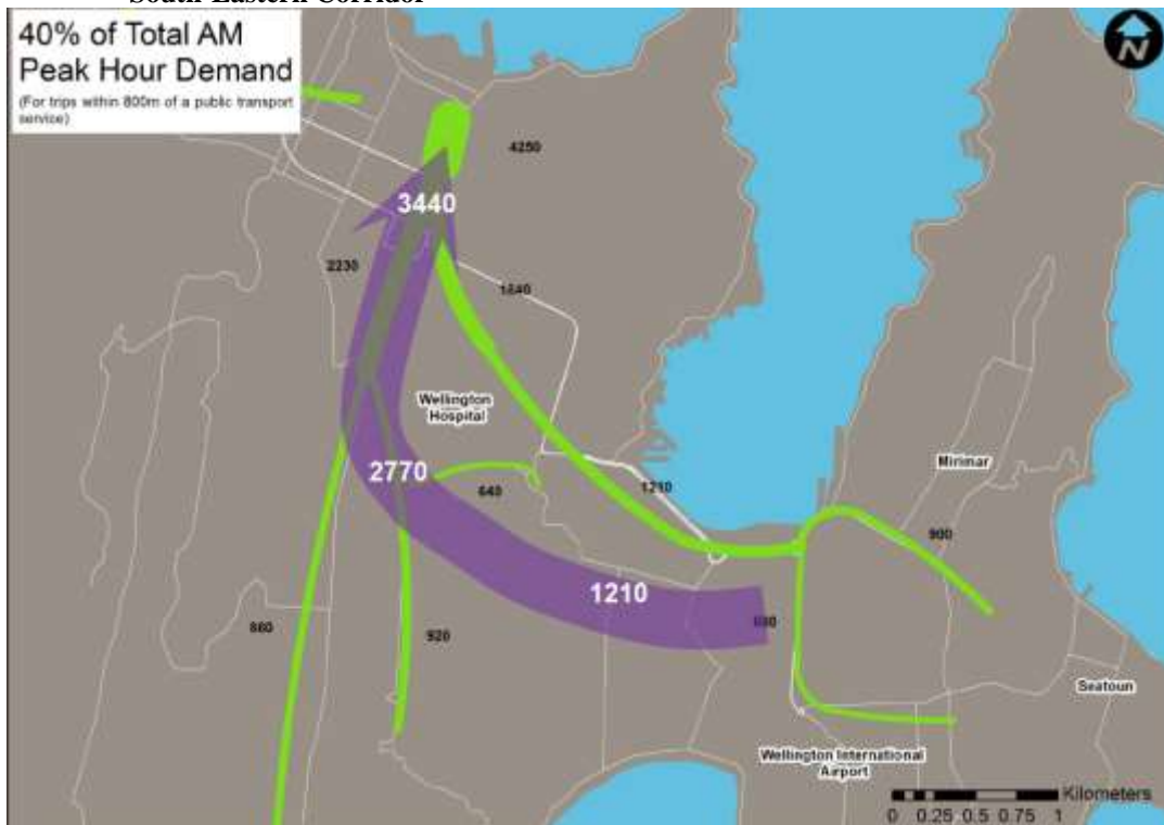
Figure 6.3 AM peak 2031 – 40% of Total (Car and PT) Peak Hour Person Demand, South-Eastern Corridor
