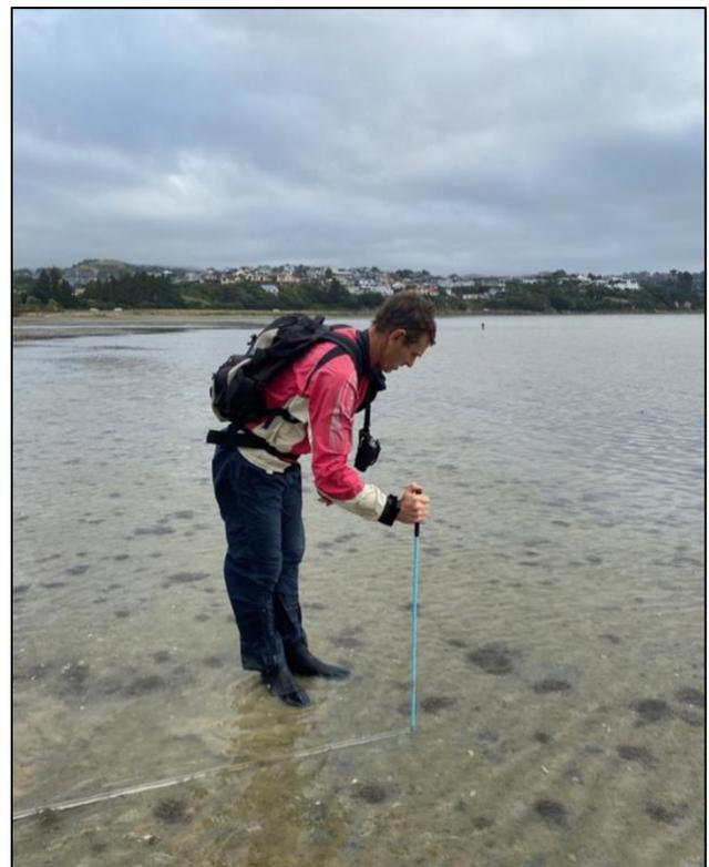
Measuring sedimentation at Site B, Pāuatahanui Inlet
