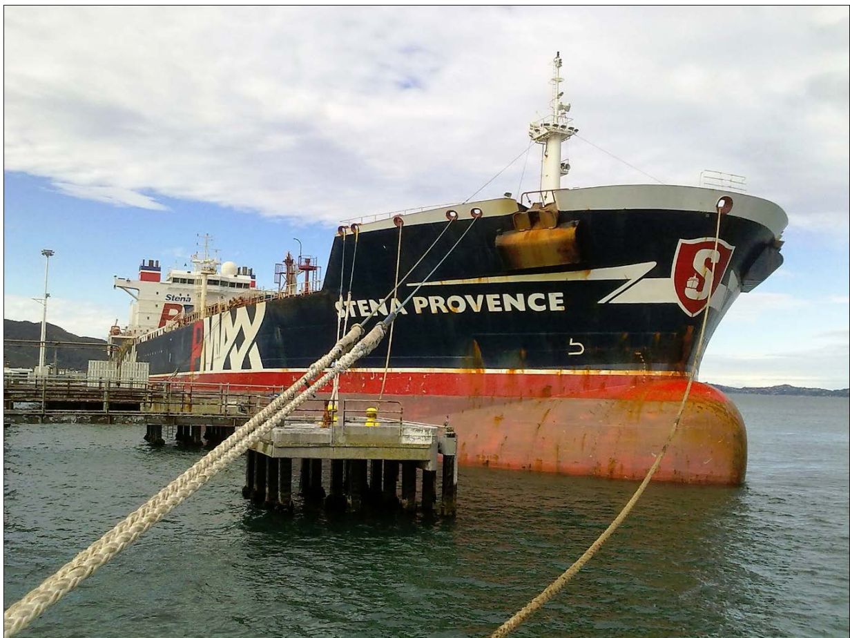
Figure 25 : Tanker Alongside Seaview Terminal – 36,168 GT 183m Length, 40m Beam
