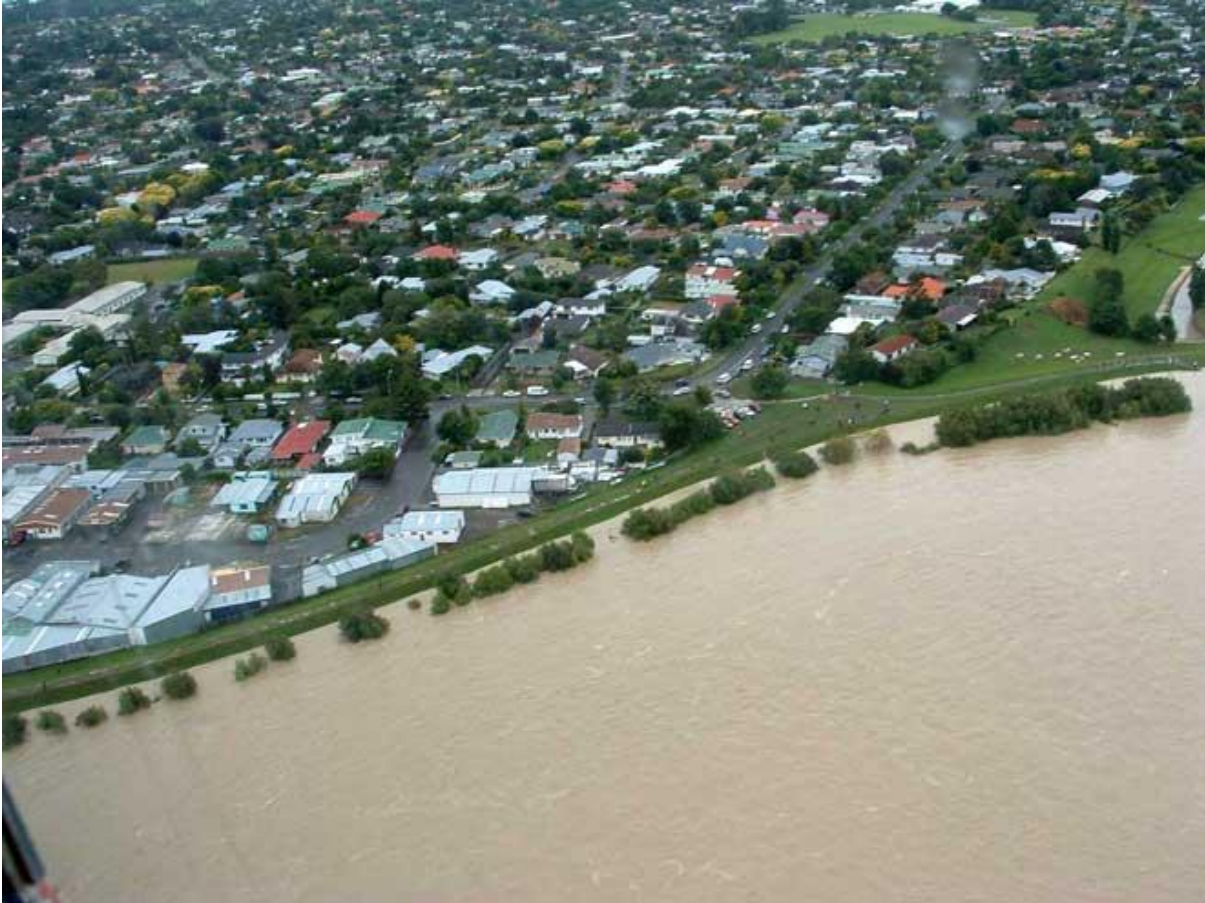
Figure 4.1: Stopbanks protected Palmerston North from inundation during the 2004 Manawatu River flood event. Source: teara.govt.nz
