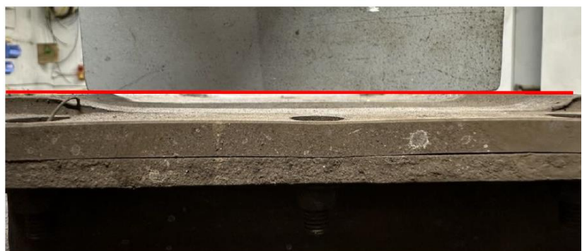
Worn wear liners with a very rough finish. Normally they are smooth and evenly worn
