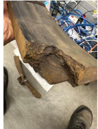
Brake blocks from myriad carriages; the failure mode is new
