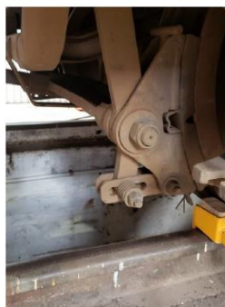
The bogies on SW3394 show much less evidence of fretting
