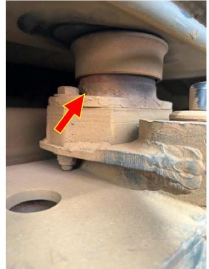
Red-coloured side bearers being found across the fleet. The red is indicative of iron fretting
