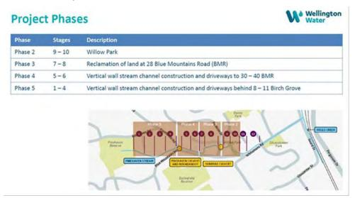
Figure 1: Phase location plan.
