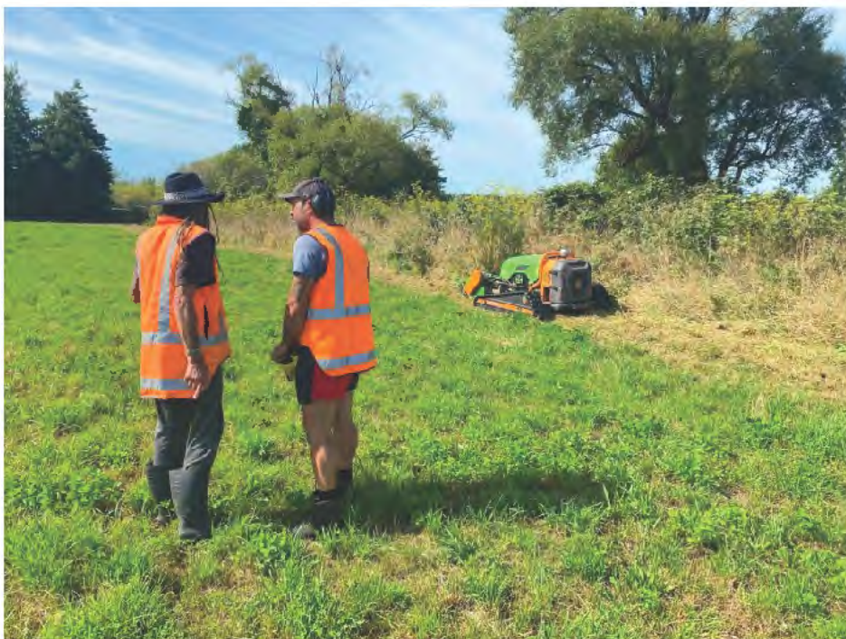
Photo1: Robotic mulcher at work
