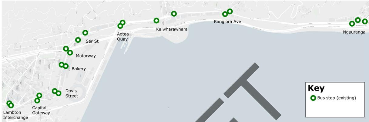
To understand the effect of the bus stop locations catchment modelling was undertaken using a maximum 400 metre buffer. Figure 2 shows the existing bus stop catchments on Thorndon Quay. It shows that some of the existing bus stops are closely spaced and have a degree of overlap in the catchment areas they serve. This is likely to be creating unnecessary delays to bus services by stopping too frequently as bus stops are located too close to each other.
